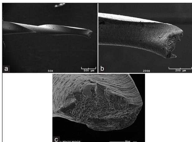
**Figure 2:** Scanning electron micrographs of (a) A size 15, 0.05 taper Mtwo instrument showing fracture (original magnification  $\times 50$ ). (b) Longitudinal examination of the specimen in A (original magnification  $\times 200$ ). (c) Fracture surface of the same specimen separated because of torsional fracture (original magnification  $\times 215$ )
